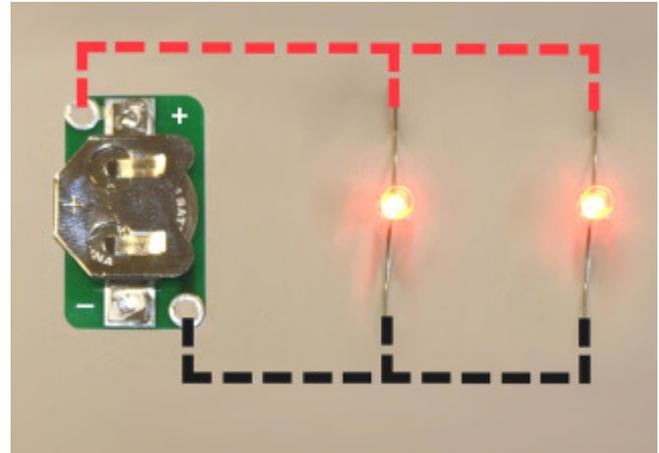
The basic sewable LED circuit is very simple and created by placing the LEDs in parallel with the battery. This is shown in the circuit diagram above left.
