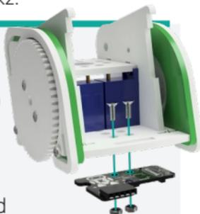
**NOTE:** Make sure you use the board the correct way up, with the larger Kit robot visible from below and the pins pointing out of the front of the :MOVE mini.
