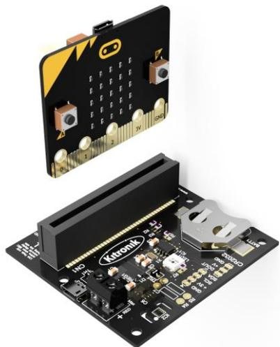
**Inserting a BBC micro:bit:** To use the RTC board, the BBC micro:bit should be inserted firmly into the connector as shown in the diagram to the left.
