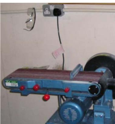
Where the pips have been cut out there is a small amount of board left over. A handful of boards are collected together and placed on to a belt sander to remove the extra material and level a flat edge.
