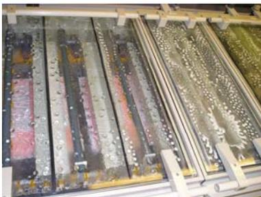
This is the same machine, in this image you can see the various wash tanks, each one in the process is slightly cleaner than the last one.
