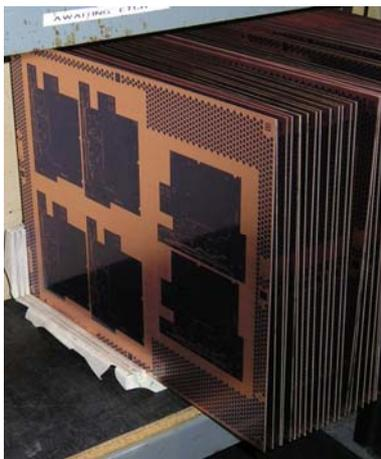
The process described above has been carried out on these boards. They now only have the protective film where the blue sections are. Unfortunately because this process takes place in a dark room there are no images, however the result is clear to see.
