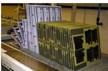
These boards have been etched and are now on an automatic conveyer, where they are stacked up waiting to go into the next machine.
