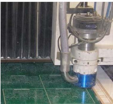
Once secured into a stack these are placed on to the routing machine. This cuts around the outline of the boards, just leaving 'pips' holding the boards to the panel.
