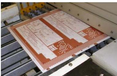
Finally the board exits the cleaning process with all the blue film completely removed.
