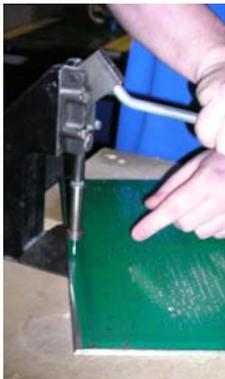
The panel is now finished, however this contains lots of separate PCBs that need to be split up. In the rim of the panel a number of production holes were drilled at the start of the process. These are now used to rivet a number of boards together.
