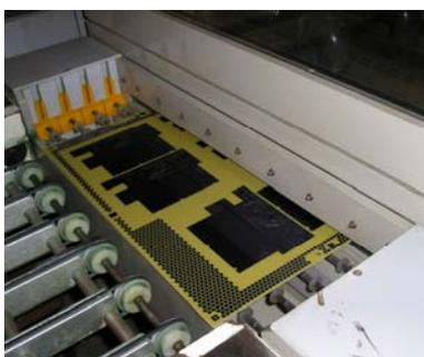
When the board comes out of the etching tank the copper has been removed. Where there was copper there is now just the yellow board. The sections that have copper remaining are still covered in the blue film.
