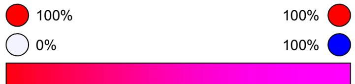
If a standard LED is turned on and off very quickly, say 100 times every second then as far as the human eye is concerned it looks like it is constantly on. If the amount of time the LED is on for is the same as the time it is off for then it will be on for 50% of the time and 50% of its full brightness.
